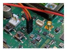
7. When finished the power button cable assemble should look like this:
