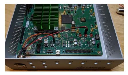
8. Connect the fan cable to J44 as shown in the figure and secure the fan cables and power button cables together with the provided zip tie:
