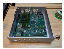
3. If not already done, install the fan assembly into the enclosure base
