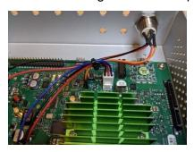
9. Connect all of the SMA to MCX cables to the enclosure, then to the AIR-T, one-by one until all 9 cables have been installed.
