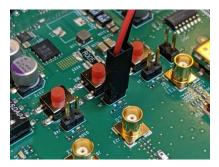
6. Connect the Red/Yellow cable to CR2 with the Red lead connected to the dot on the solder mask.
