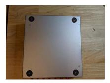
12. Place the mounted and assembled AIR-T enclosure upside down in the external housing and insert the aluminum standoffs between the enclosure and external housing.
